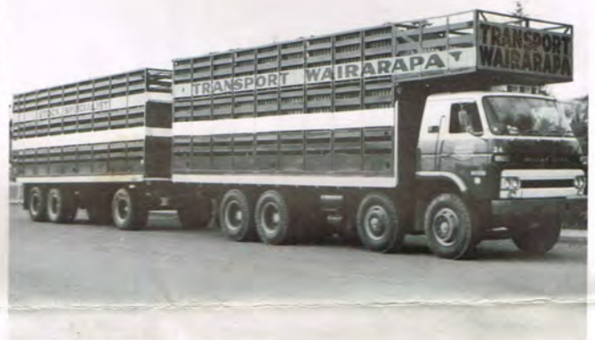
This modern three deck stock transporter can carry between 650 and 700 fat lambs or 33 to 36 bullocks.
