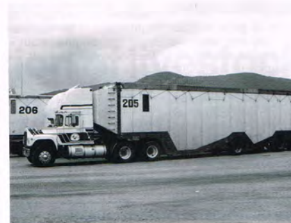
4. This 6 axle semi Chipliner is a little different. The first axle on the trailer is steerable and also lifts to aid manoeuvrability.
