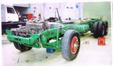
The completed rolling chassis
